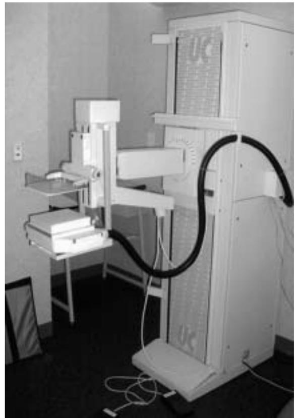
FIGURE 1. Prototype gamma camera mounted on a modified mammographic gantry.
